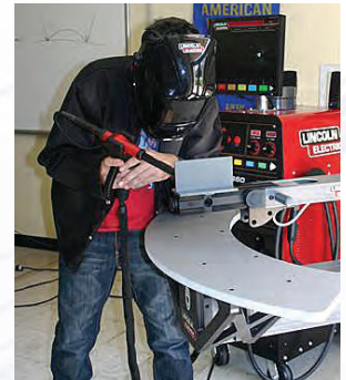
Aiken Technical College student Chris Kunka practices his welding skills on a virtual welding machine during class
