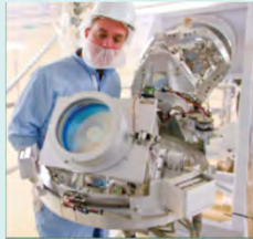
A National Ignition Facility technician examines a damage inspection instrument used to assess the optics in the target chamber.
