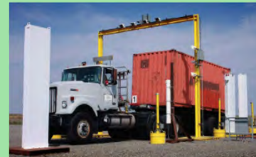
A container with naturally occurring radioactivity processed through a radiation portal monitor as part of NNSA's Second Line of Defense Program.
